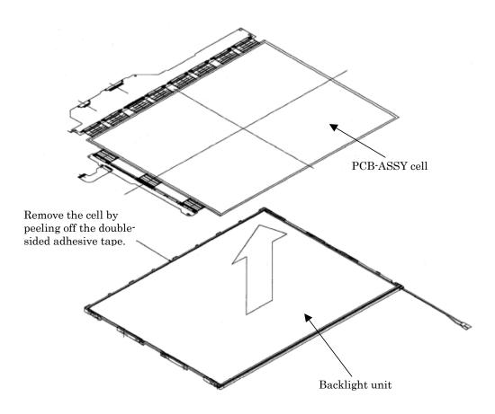
Figure 4-55 Replacing TMD fluorescent lamp (WXGA) (5)
